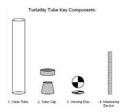
Figure 1: Turbidity Tube Key Components
