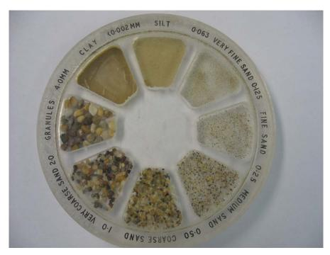
Figure 2: Sediment sizing wheel
