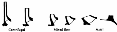
EFFECT OF SPECIFIC SPEED ON IMPELLER SHAPE [JONKER 1995]
