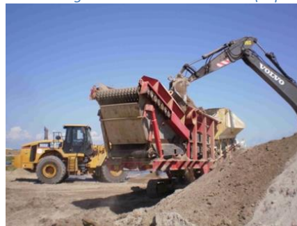
Figure 2. Pretreatment of the sediments: dewatering of sediments by lagooning (left), on site pre-treatment of lagooned sediments with a CSA additive.
