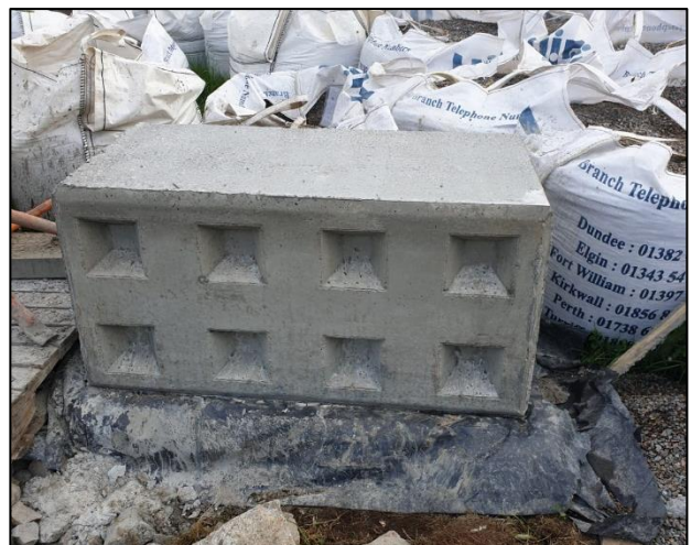
Figure 5. Concrete block manufactured from Laggan aggregate.
