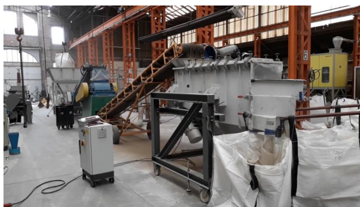
Figure 3: line prepared for sediment grinding (equipment in blue) and sieving (white equipment in front).
