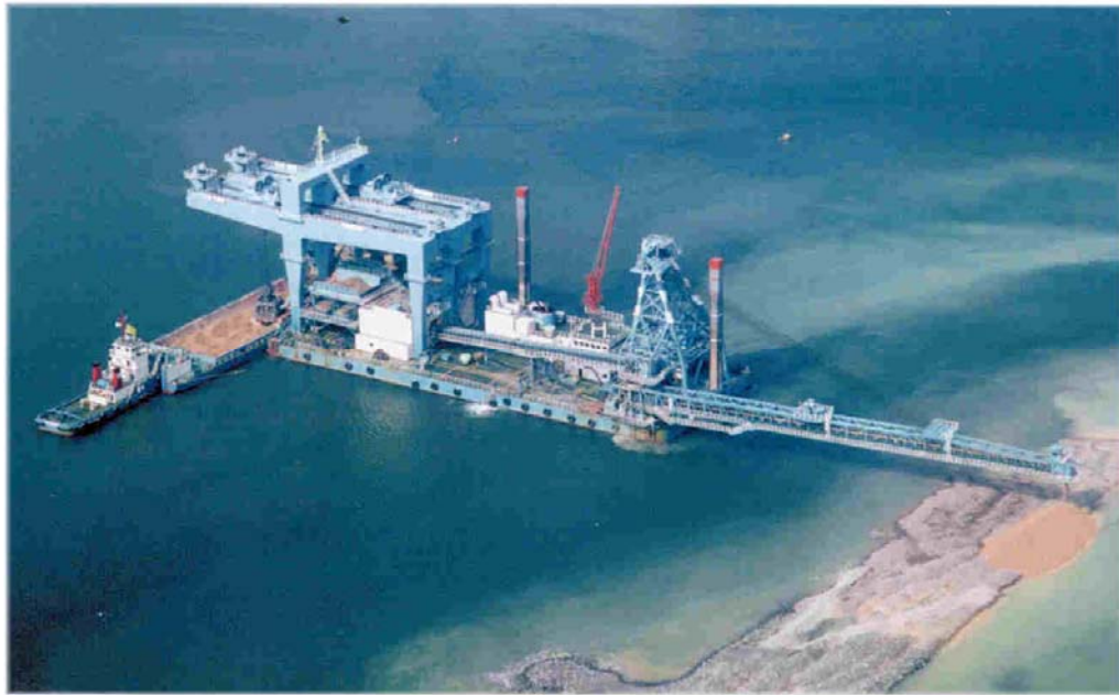
Figure 7- 3 Grab bucket reclaimer
