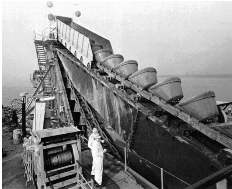
5. 10 Bucket ladder of the demountable bucket dredger "Big Dalton"
