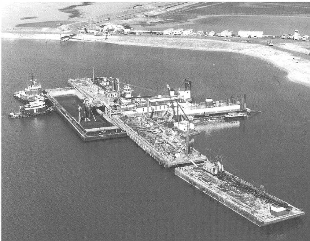
Figure 5-24 The CSD "VICKSBURG" converted to a Barge Unloading Dredger
