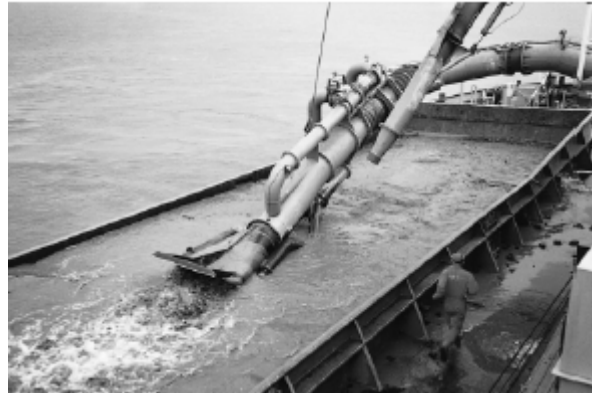
Figure 5-9 Suction mouth and pipe
