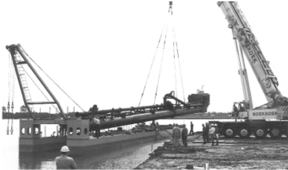
Figure 4.36 View on ladder with pump for a PSD
