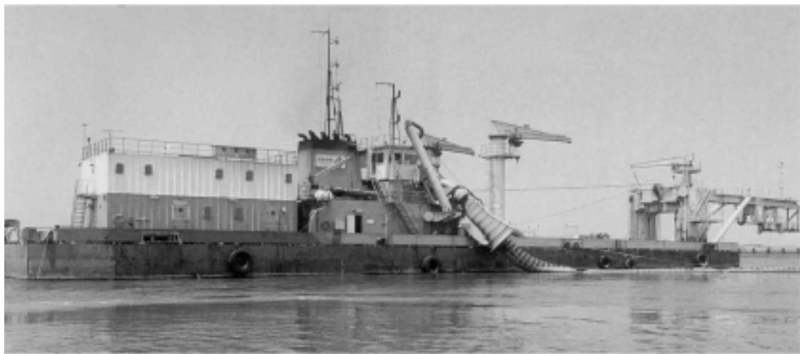
Figure 4. 38 The sea-going PSD AURORA with the discharge pipeline connected on starboard
