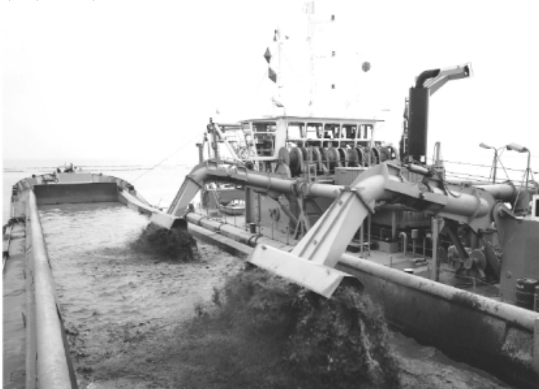
Figure 4. 40 barge loading with movable sprayers
