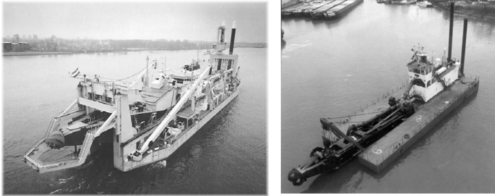
Figure 3. 11 Different cutter dredgers with ladder above waterlevel
