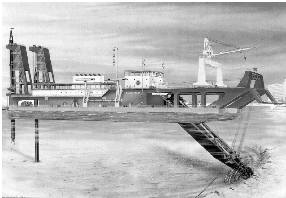
Figure 3. 1 The "Mashhour", at present the biggest cutter suction dredger in the world,
