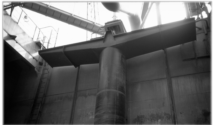
Figure 2-101 Adjustable overflow over the full width of the hopper
