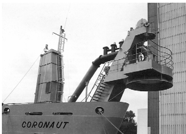
Figure 2-10 Pump ashore connection
