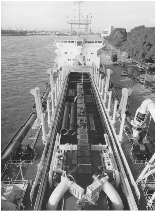
Figure 2-90 TSHD with one delivery line
