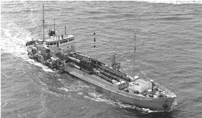
Figure 2-91 TSHD with 2 delivery pipes
