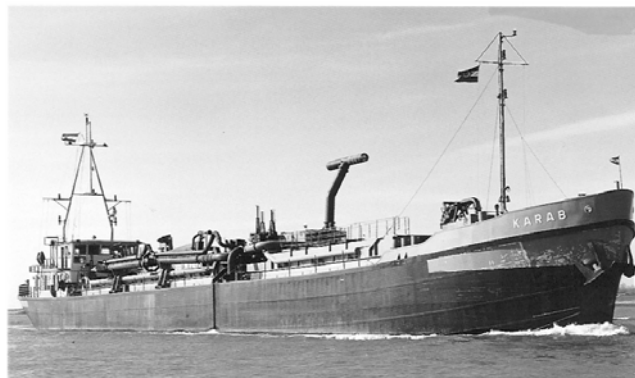
Figure 2-145 Trailing suction hopper dredger for inland waters
