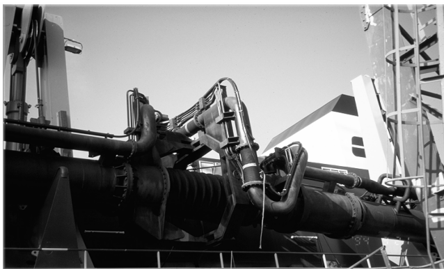
Figure 2-78 Jet pipeline passing the universal joint
