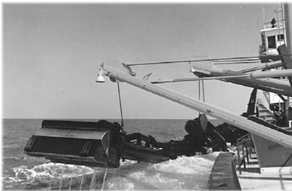
Figure 2-35 Draghead with jets (not working)
