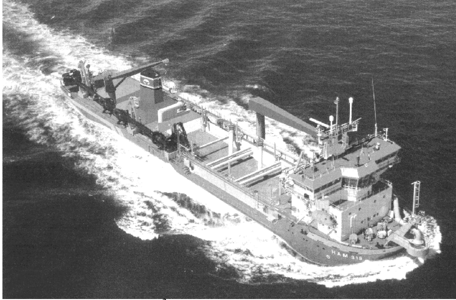
Modern 9000 m 3 Hopper dredger with one dredge pipe
