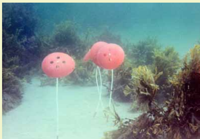
Near bed flow and sediment transport patterns can be investigated by using seabed drifters which are released at the disposal site.
